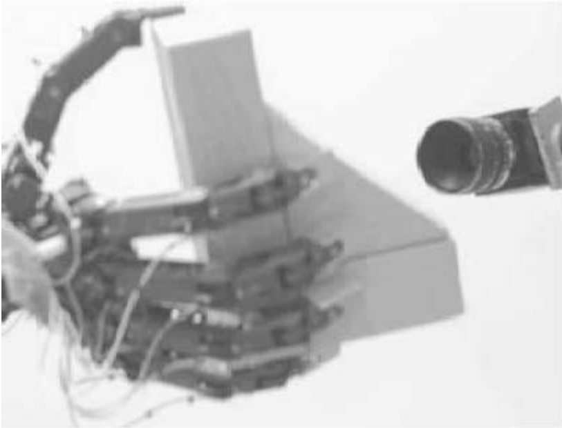
Fig. 7.13. The Anthrobot five-fingered hand holding an object in the field of view of a fixed camera. The contact data obtained from tactile sensors mounted on the fingertips is fused with the processed image data obtained from the camera, to estimate the position and orientation of the object.
